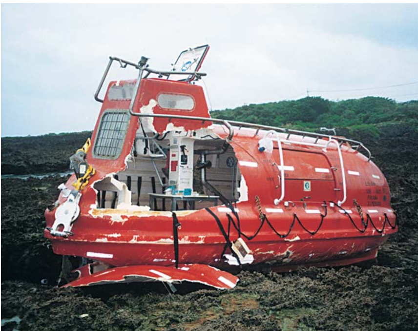
This lifeboat released itself from a vessel, fortunately without anybody on board. It was found on a coral reef two weeks later.
